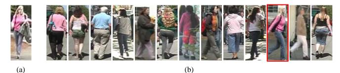
Figure 1. A query image(a) and the gallery images with sorted order(b). These results are generated using HSV color histogram applied in 6 horizontal non-overlapping strips of person images and the similarity score is computed by Bhattacharyya distances. Note that the query is wearing pink but the many candidates who are not wearing pink are ranked higher than the true match.
